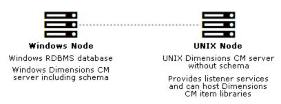
A remote database server is an RDBMS with a Dimensions CM schema installed. To enable network connections between the nodes the remote database server must be running the TNS listener. You may also need to set up an Oracle Net Service Name on the local node to access the Oracle database server. For details, see "Set up a local Oracle Net Service Name" on page 52.
