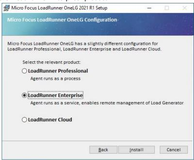
In SaaS, for most installations we highly recommend choosing "LoadRunner Enterprise". This leads to installing load generators as a service, providing multiple advantages, including permanent and immediate availability (hosts listed as "Operational" automatically) and the resulting reliability of the setup.
