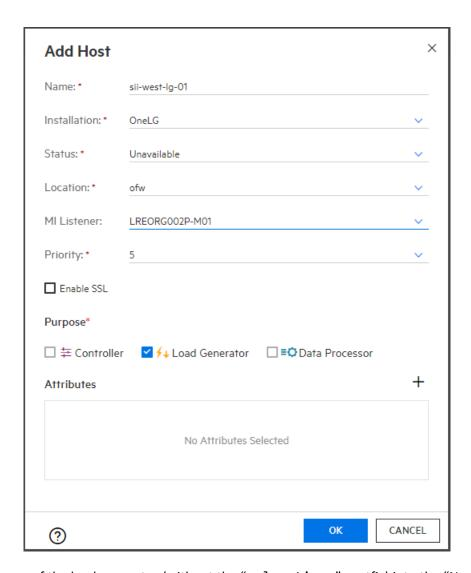
Enter the name of the load generator (without the "\_<location>" postfix) into the "Name" field. In our example, enter "sii-west-lg-01". It is important that the string entered here will exactly match the local machine key that will be entered into the host's configuration upon installation, without the "\_<location>" postfix. Please follow the SaaS naming policies described in the next chapter, "Policy for selecting valid load generator names", and "Policy for selecting valid location names".
