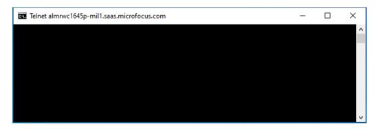
Then the firewall is open from the load generator to the MI Listener on port 443, as it needs to be for direct communication. You can click the "X" close icon to close the window and log off.
