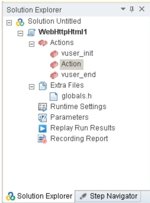
This tab provides you structured access to the various parts of a Vuser script, as well as to a number of files that are associated with the Vuser script.
