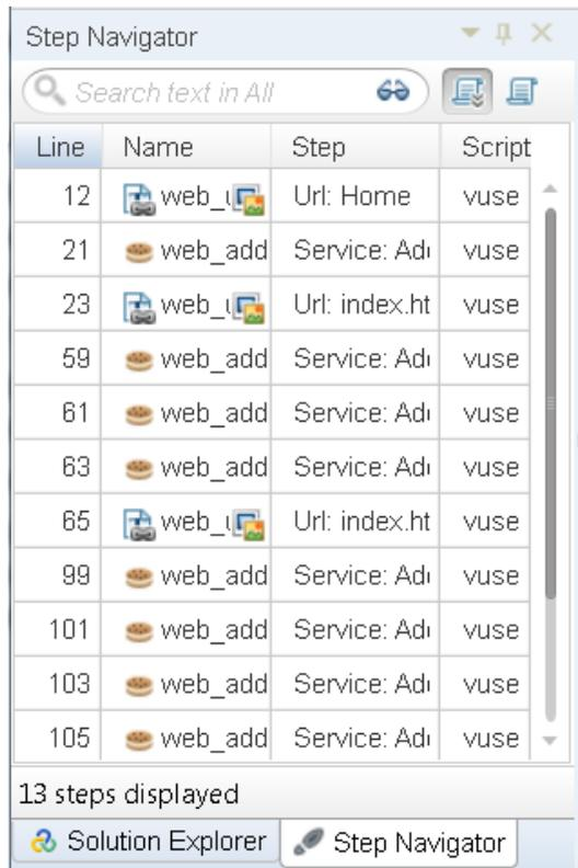
The Step Navigator displays an icon-based view of the script that lists the actions of the Vuser as steps. For each action you performed during recording, VuGen generated a corresponding step in the Step Navigator.
